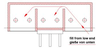
**2.2.9.** Fix foam damming on the end of the bedplate or under the bedplate. Do not fix metal front damming plate at the end; you will get cracks or voids.
