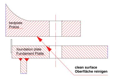
2.2.7. Flexible damming is inserted between the bedplate and foundation to form liquid tight sides for the moulds or dams. Make sure the damming is firmly in place, and cannot collapse or leak. The EPOCAST 36® exerts a surprisingly strong pressure on the lower edge of the damming. So take extra care when forming dams.
