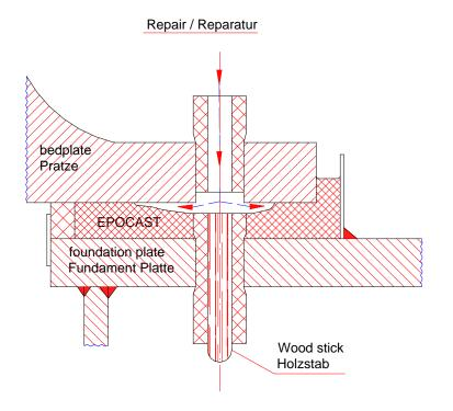
**2.8.2.** Sometimes a vertical crack occurs running into the bolt hole. This can be left, but for aesthetic reasons it is usual to grind out the crack to about 30 mm and pour in new **EPOCAST 36**® to repair the crack.
