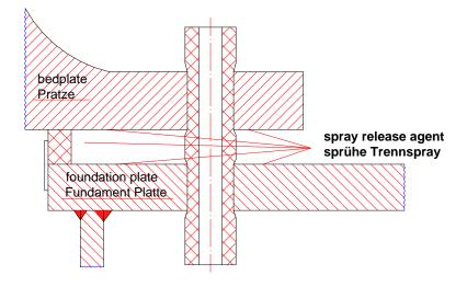
**2.2.12.** For generators, deck machinery and small units you may apply a thick coating of thick high melting point grease to the holding down bolts before inserting them. These bolts should only be hand tight. If chock thickness exceeds 50 mm then follow instructions for larger units in the next paragraphs. Where possible use foam plugs in preference to wood plugs or bolts.
