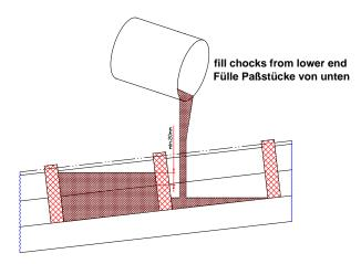
**2.3.10.** Until the resin sets keep a careful watch for leaks. During setting **EPOCAST 36**® will be drawn into the chock from the overpour. Where chocks are large this reservoir may need to be
