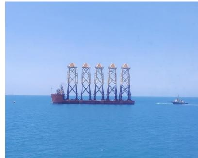
on the Ducorit S5R as part of the total system. The Ducorit S5R system was critical to connect all 21 jackets with approximately 1,100 metric tonnes for the site.
