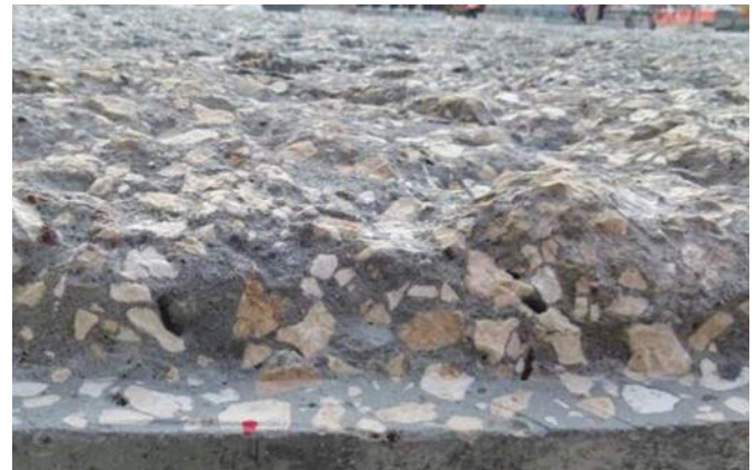
FIGURE 1: CONCRETE SURFACE WITH APPROXIMATELY 50% FRACTURED, COARSE AGGREGATE VISIBLE
