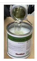
7. Slowly pour the entire contents of the Part B (Hardener) can into the Part A (Resin) can
