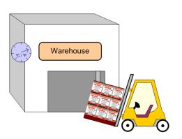
3. Pre-condition the entire kit, including the Resin, Hardener, and aggregate, as well as the application area.
