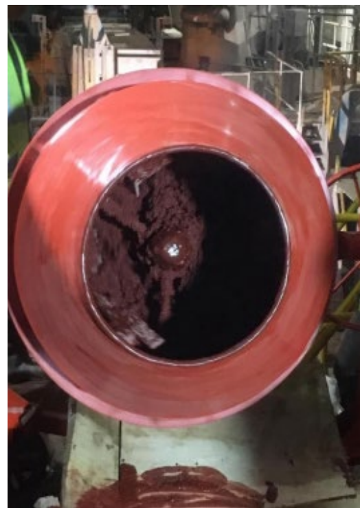
Chockfast Red mixed in-house
