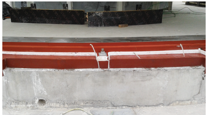
Anchor bolts aiding in the transfer of vibration
