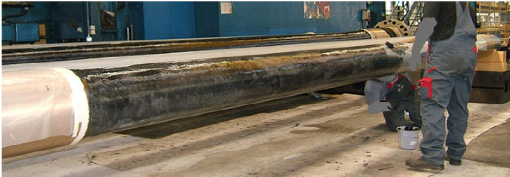
... and wrap immediately a glass silk tape in a spiral manner around the shaft before the hardening process of **WBD** starts. The edges should not overlap.
