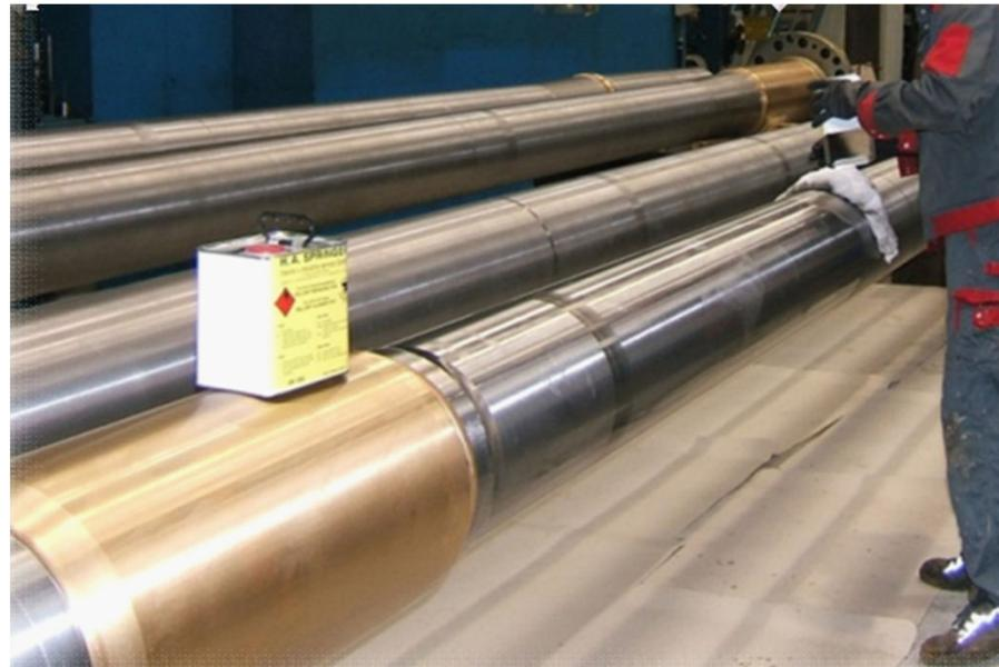
... mix the component “**WBS**” resin and hardener to a homogeneous mixture with our special mixer ...
