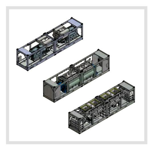
Increase efficiencies through crane-free big bag loading by using the on deck hopper and elevator system.
