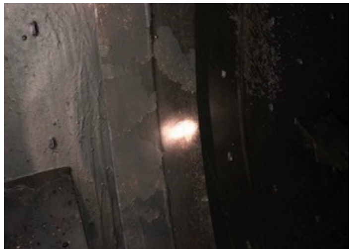
Devcon Brushable Ceramic Coating after 6 years
