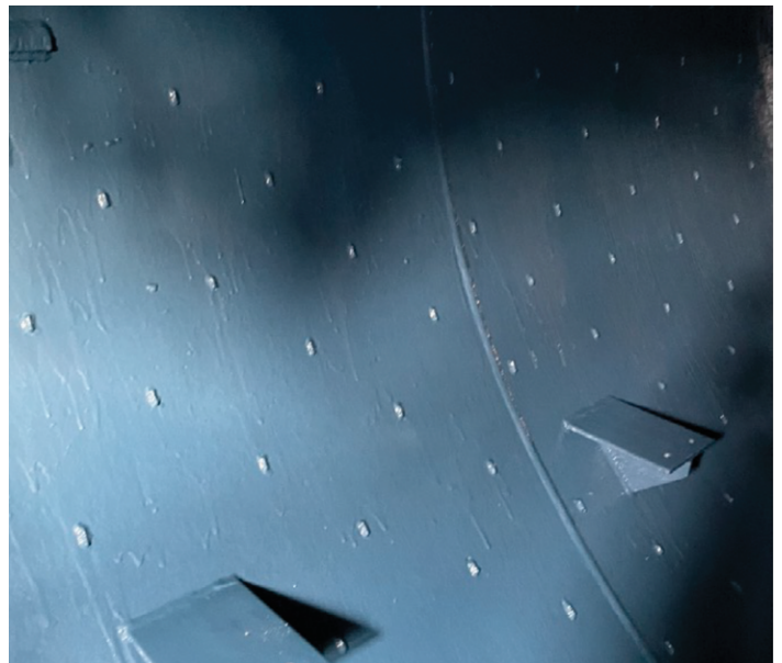
Recoated with Devcon Brushable Ceramic Blue
