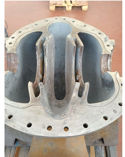
Devcon Fine Load applied to abraded pump internal walls
