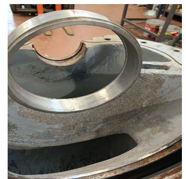
Devcon Fine Load applied to abraded pump internal walls
