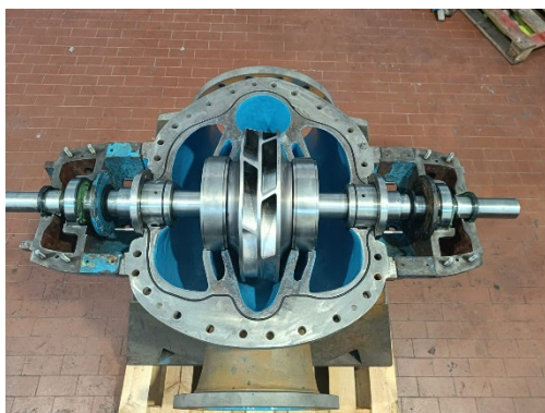
Devcon Brushable Ceramic lining interior walls
