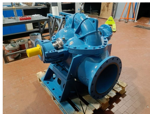
Pump and housing assembled and ready to go
