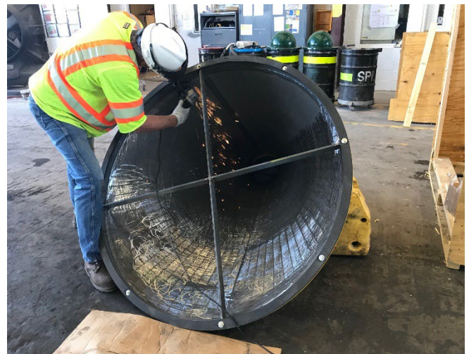
Surface preparation of gold mine drill cone
