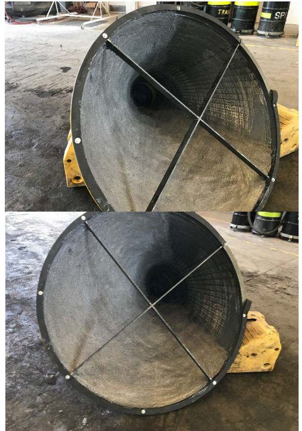
Drill cone coated with Devcon DFense Blok
