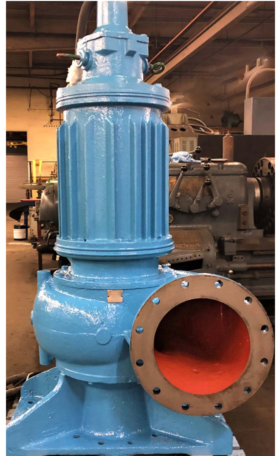
Pump Refurbished with Devcon EZ-Spray Ceramic
