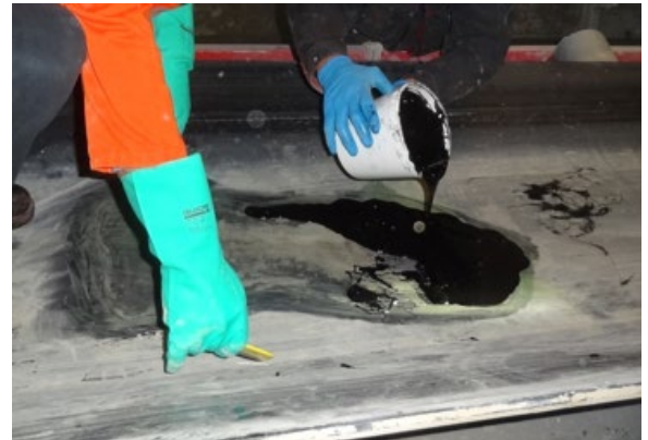
R-Flex being poured onto damaged transport belt area
