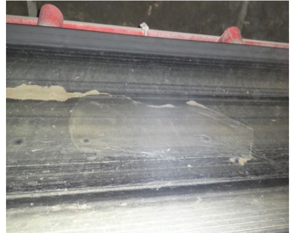
Devcon R-Flex repair system application
