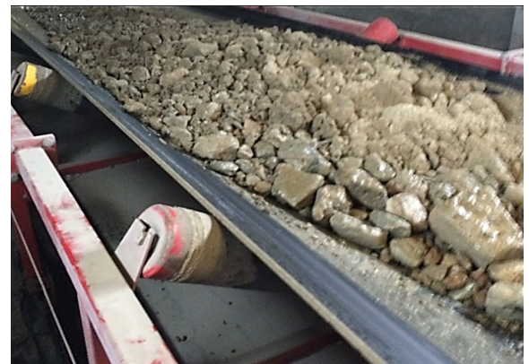
Limestone transported via conveyor belt
