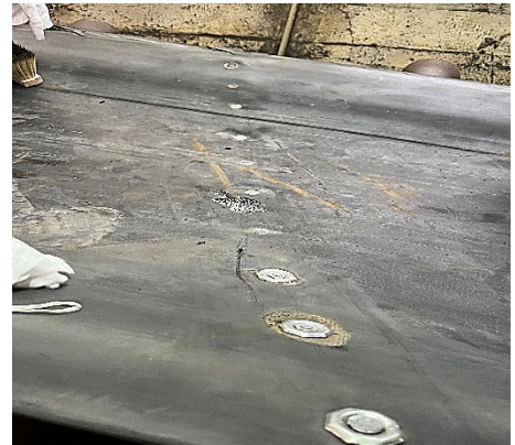
Damaged conveyor belt
