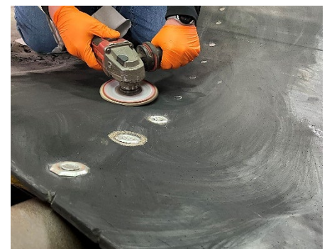
Surface abrasion with abrasive wheel
