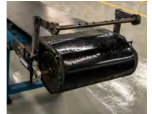
After: R-Flex® Clip Repair
