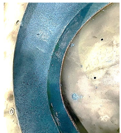
Close up of pump interior coated with Devcon Wear Guard 300RTC
