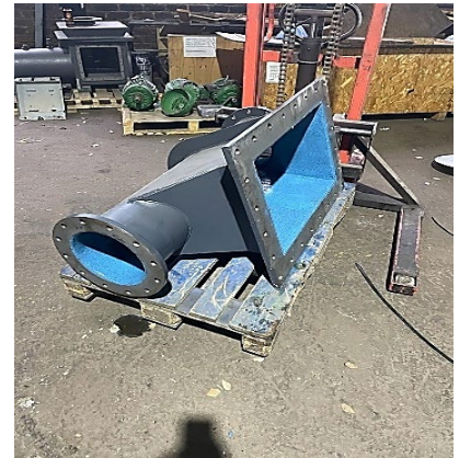
Slurry transfer chute protected with Devcon Wear Guard 300RTC
