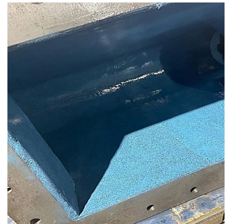
Devcon Wear Guard 300RTC in transfer chute
