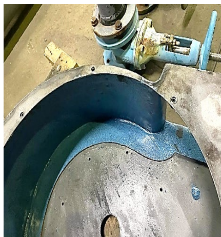
Spare pump part coated with Devcon Wear Guard 300RTC
