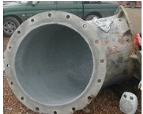
Fully repaired transfer pipe
