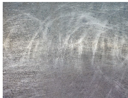
Surface preparation – abrading metal
