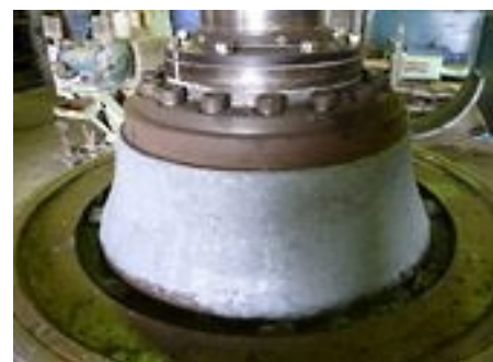
Vertical coal mill roller bush
