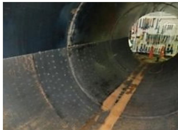
Coal dust collector facing abrasion in bottom half of equipment
