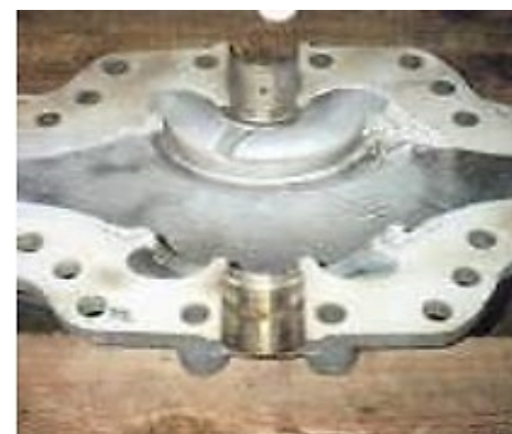
Fly pump after Cleaner Blend 300, Titanium Putty, and Wear Guard Fine Load application
