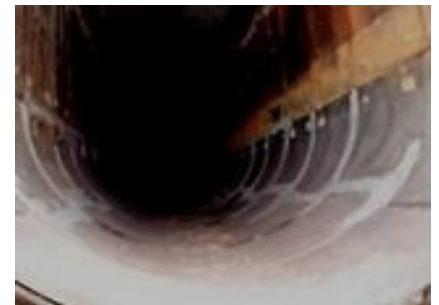
Chute coated with Devcon Wear Guard Fine Load
