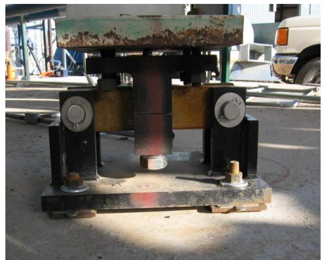
Silo loading cell
