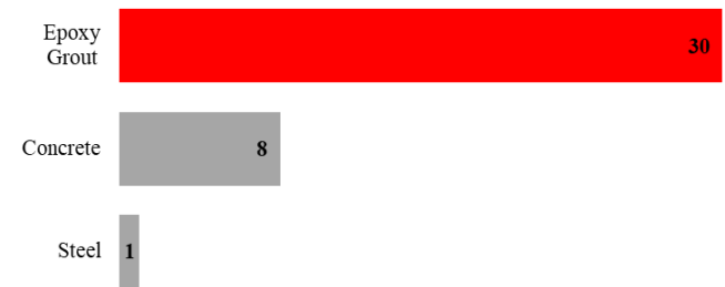
Figure 3: Vibration Absorption Capacity of Common Foundation System Materials
