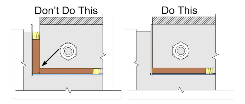
Do NOT pour EPOCAST 36 around a corner. It will always lead to cracking because the corner acts like a wedge.
