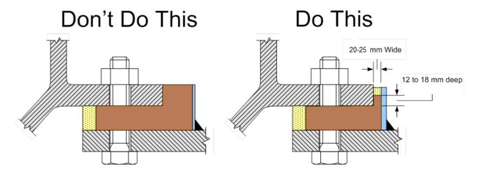
The **EPOCAST 36**® in the overpour area must remain cool and liquid to feed material back under the engine bed if needed. To do this, the overpour must be small and kept cool with a heavy metal front dam.
