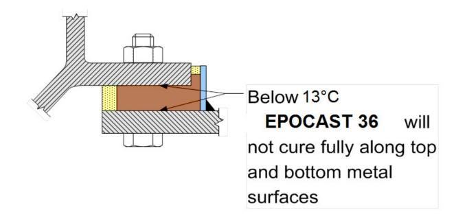
**EPOCAST 36**® resin can be re-awakened and will restart its curing process when its temperature reaches 13°C.
