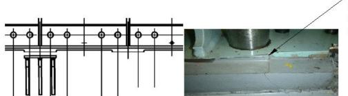
Sharp corners protruding into the EPOCAST 36 act like a wedge and cause the EPOCAST 36 to crack
