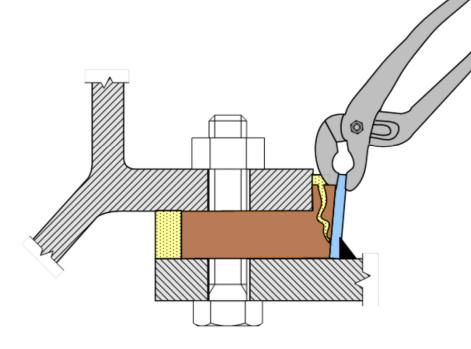
Wait until the **EPOCAST 36**® has cured completely before removing the front metal dam or you could break the chock.
