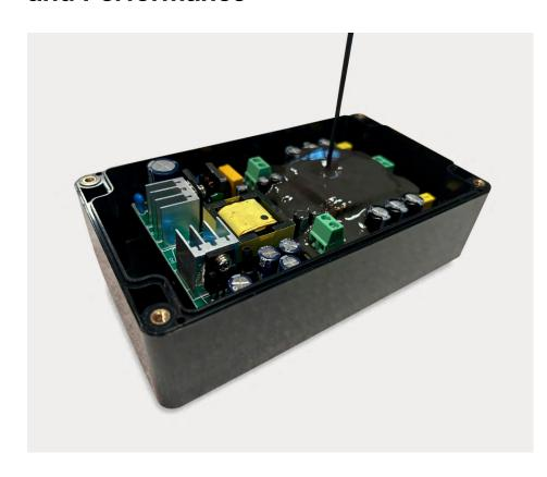
Insulcast RTVS 27 is a low viscosity reversion resistant RTV silicone used for the manufacture of power supplies, sensors, controllers, and other electronic insulation applications. Insulcast RTVS 27 combines the virtues of low temperature flexibility, excellent electrical properties, high temperature resistance, and easy removal for component replacement or repair.
