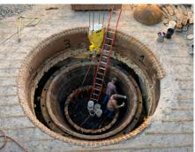
Devcon Korrobond 65 is a high performance backing compound for use in rock crushing equipment including gyratory and cone crushers. This proven shock absorbing compound extends the life of crusher equipment by preventing common issues such as leaks, corrosion, and loosening thereby increasing plant productivity.
