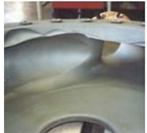
Sandblasted coal ash transfer pump
