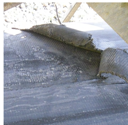
Before Repair: Large tear in belt due to rocks getting caught under the scraper blade.
