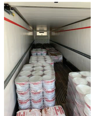
Figure 11: Conditioning of Epoxy Grout Components
