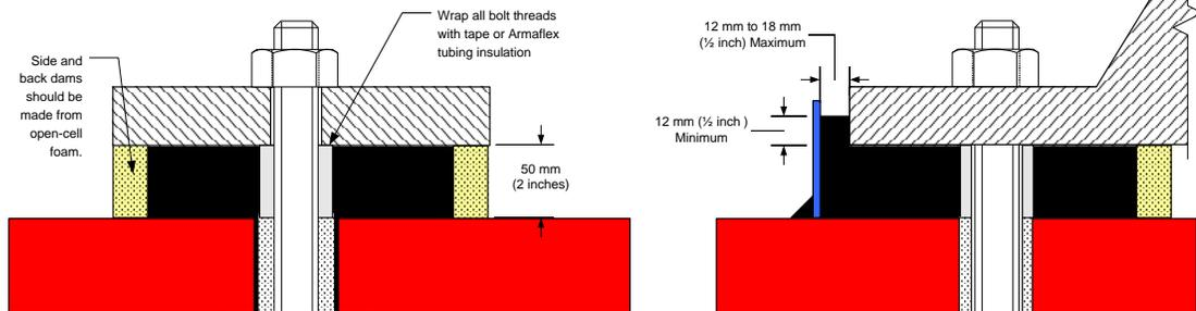
An aerosol release agent, as supplied by ITW Performance Polymers, should be sprayed into each prepared chock area. Only spray enough release agent to provide a fine misting of the chock area without puddling.
