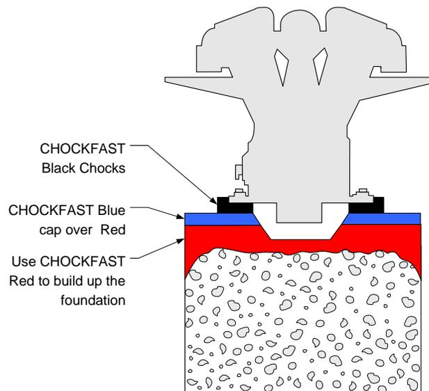
Use grout as soon as possible after mixing. CHOCKFAST Blue pot life is approximately 35 to 50 minutes at 70°F (21°C). Cure time for CHOCKFAST Blue is as follows:
