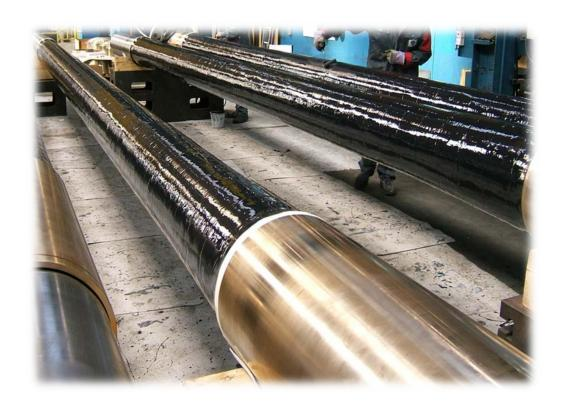
Apply a 2<sup>nd</sup> and if necessary a 3<sup>rd</sup> layer **WBD** (after curing of each single layer) in order to achieve a proper and good looking surface.
