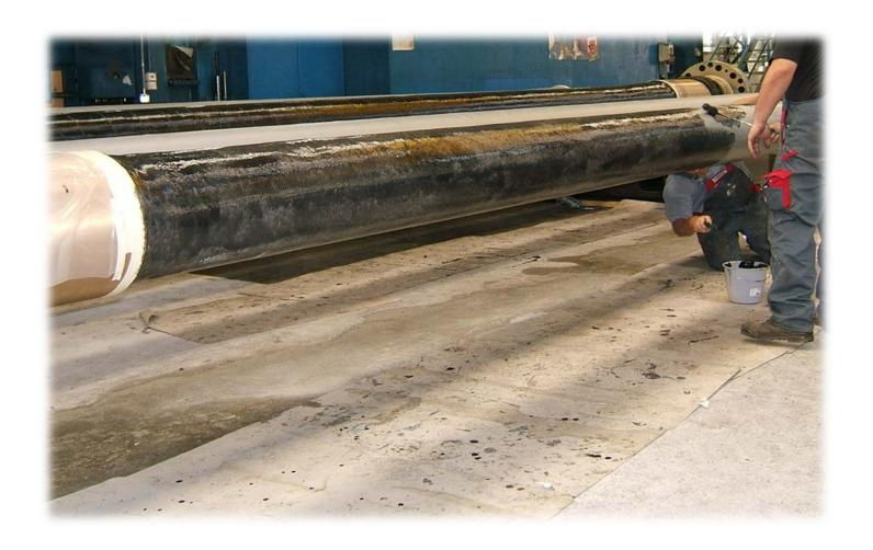
... and wrap immediately a glass silk tape in a spiral manner around the shaft before the hardening process of **WBD** starts. The edges should not overlap.
