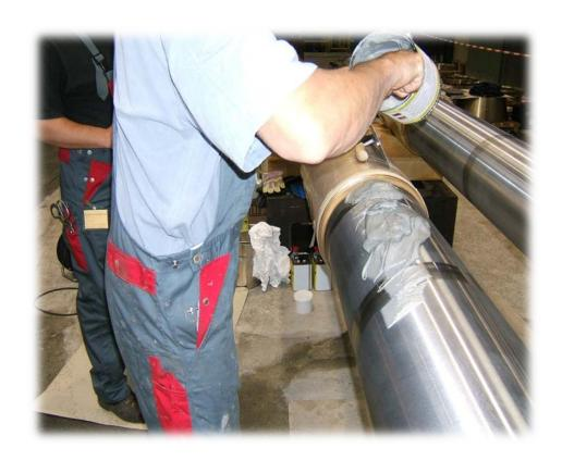
...and dispense equally by using a serrated pallet-knife (4mm) in order to achieve the required thickness of layer. Let it cure.
