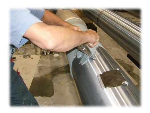
Apply an additional thin layer **WBS** in order to achieve a smooth surface. Dispense the material equally with a normal spatula / pallet knife.
