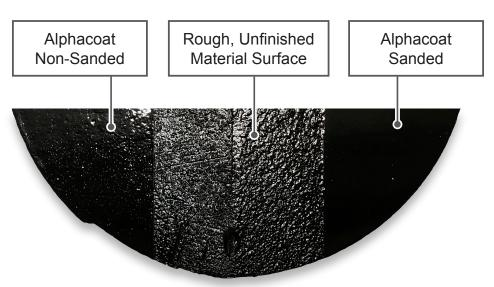
Alphacoat 1700 is a sprayable polyester based filler. It creates a sandable finish on iron, aluminum, fiberglass and wood.
